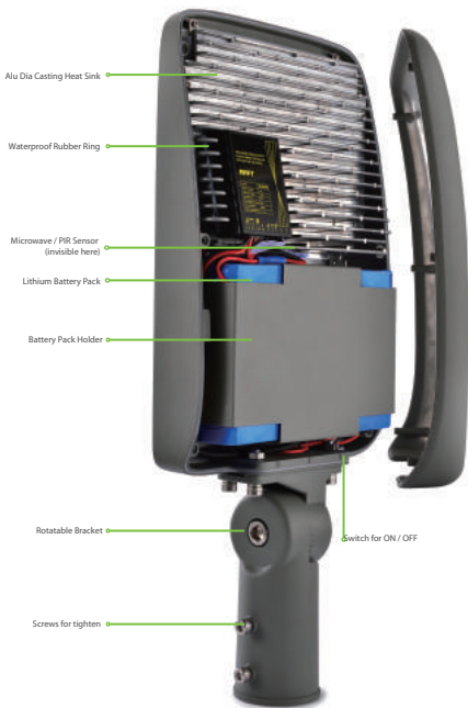
Internal structure of HELIOS solar led street light
